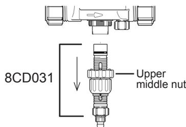
5. From the injection stem assembly (8CD031), unscrew the check valve nut (PDI056) and remove the check valve assembly (PDI006) by pulling straight down.
