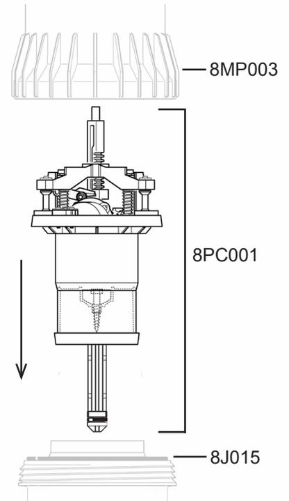
10. Take the new plunger assembly (**8PJ008**) and screw it back onto the end of the piston assembly (8PC001).
