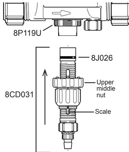
11. Take the whole piston assembly (8PC001) and reinsert it back into the body. Apply **Dosa-Lube** on bell housing o-ring (8J015). Screw the bell housing (8MP003) back on.
