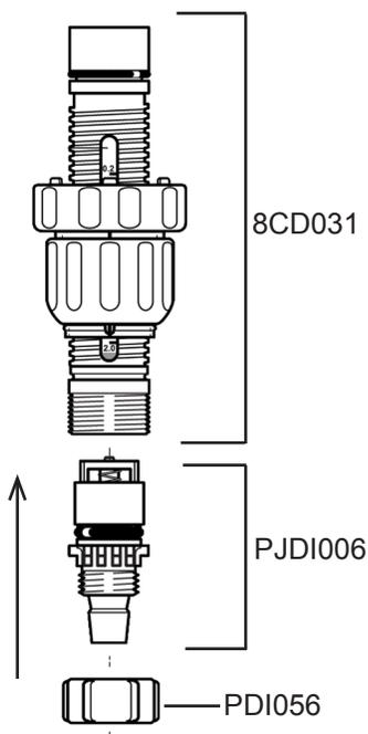
9. Apply a small amount of **Dosa-Lube** onto the injection stem assembly o-ring (8J026), then reinsert the injection stem assembly (8CD031) back into the bottom of the unit with the scale facing forward. Screw back the upper middle nut making sure the keys line up with the notches on the threaded diffuser nut (8P119U).
