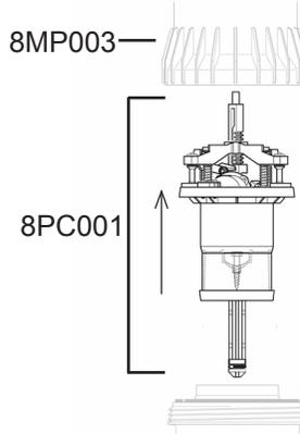
3. From the lower part of the piston assembly (8PC001) unscrew the white plunger assembly (8PJ008) and discard.
