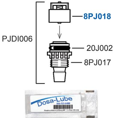
**NOTE:** Do not apply **Dosa-Lube** inside the check valve.
