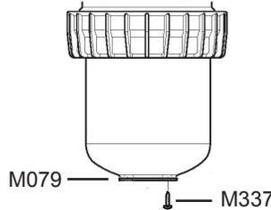
4. Remove the injection stem assembly (CD070), exposing the plunger seal (**J009**). Remove the plunger seal by squeezing the seal and rolling it off. Discard seal.
