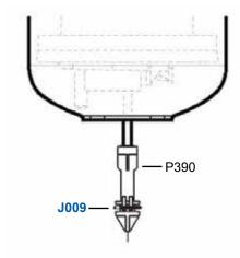
**NOTE:** Do not apply **Dosa-Lube** to plunger parts.
