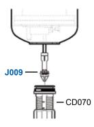
To remove seal easily without tools, squeeze it on either side to raise the seal, then slide it over the groove. Using sharp tools could damage the plunger.
