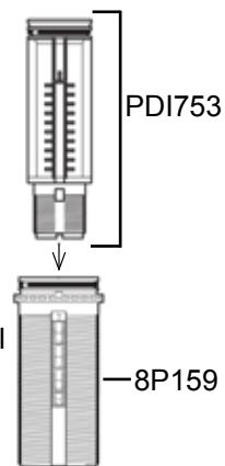
11. Slide the injection stem assembly nut (PDI702) onto the black sleeve (8P159). Then screw the adjusting sleeve (PPDI037) back onto the black injection sleeve (8P159).
