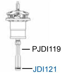
16. Insert the piston assembly (8PC002) into the lower housing (8PP010NPT), then screw the upper bell housing (8MP039) back in place.
