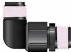
**6** Install the **Elbow** assembly at the bottom opening of the **Tee**. Make sure the **Nipple** faces to the right.
