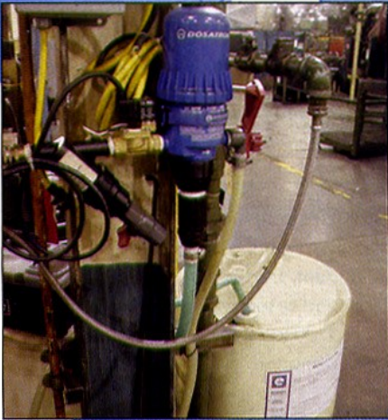
Dosatron dispensers provide on-demand, consistent coolant dilution, compensating for changes in water pressure and flow.
