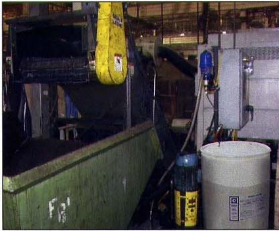
Consistent coolant sump levels are critical to maintaining proper chip flush and conveyor operation.
